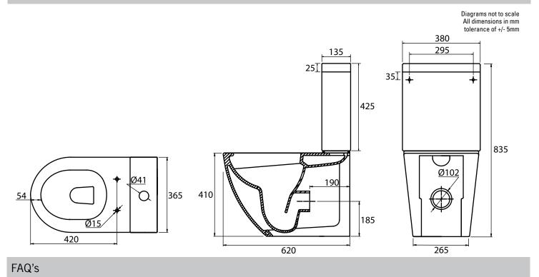
What side is the inlet valve in the close coupled WC? Bottom left of the tank.
