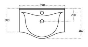
All Dimensions are in millimetres. The information contained on this page was correct at date of issue. Fitting dimensions are provided as a guide only. Some variation may occur due to manufacturing tolerances. We pursue a policy of continuing improvement in design and performance of our products and so reserve the right to change specifications without prior notice.
